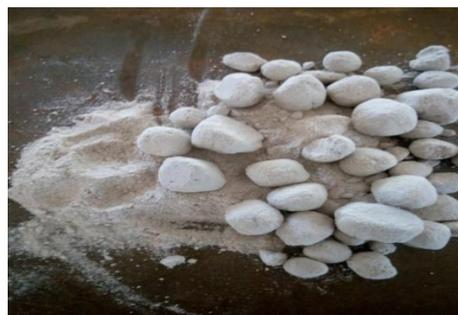
**Fig. 3. Acid activated montmorillonite clay**
