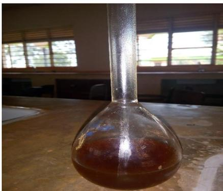
**Fig. 6. Dark brownish fuel oil produced from plastic wastes**
