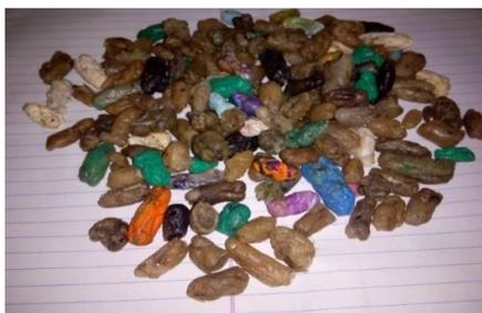
**Fig. 1. Pellets of a mixture of HDPE and LDPE plastic wastes**
