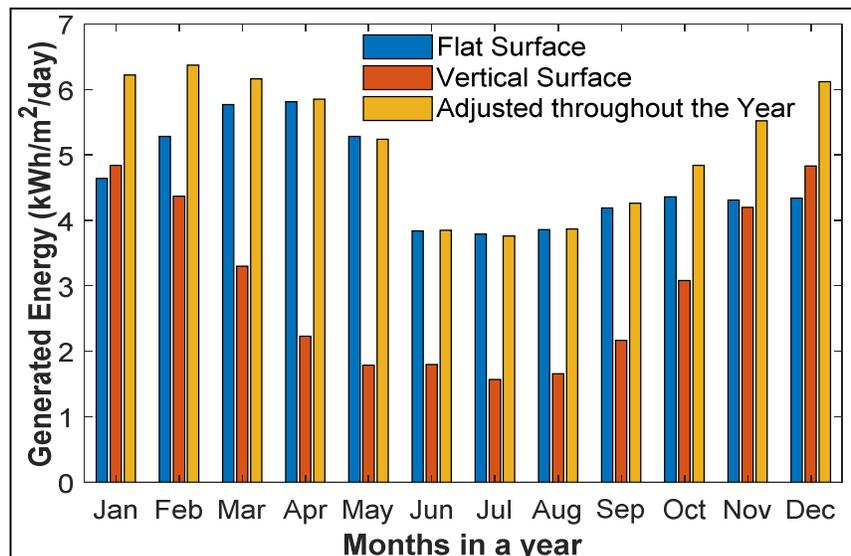
Fig. 4. Energy generated for different insulations in Cox's Bazar
