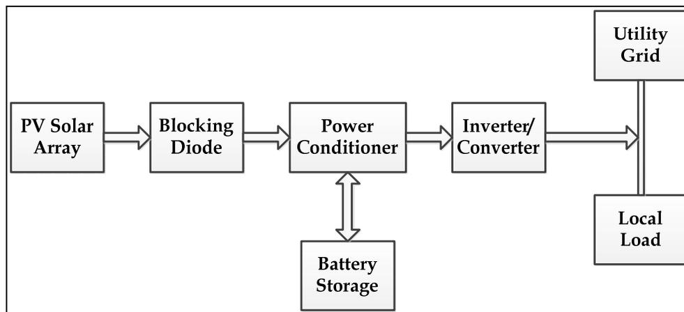
Fig. 1. Block diagram of a PV power system
